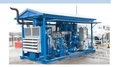
Piston and rotary vane process compressors
